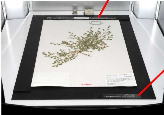
Figure 9. Proper placement of custom ruler and specimen label tag.
