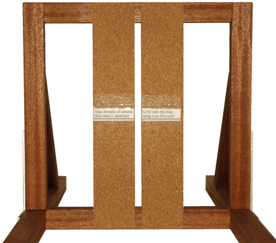
Figure 3. Vertical risers of camera mount, with cork pads attached and camera alignment guide taped into place..
