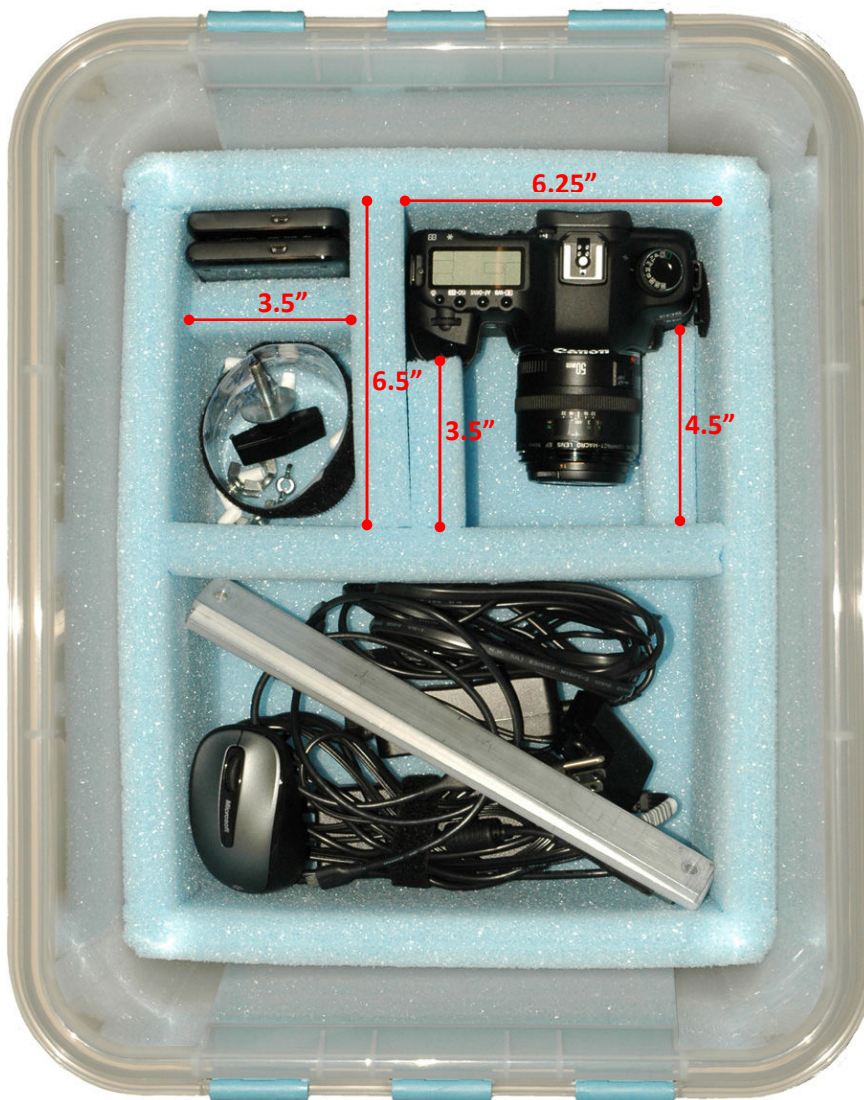
Figure 12. Storage tub with foam liners and cubbies. Measurements shown are guidelines, and should be adjusted to fit the size of your tub and equipment.
